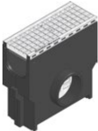
Trash box with galvanised bucket, with mesh grating MW 30/30 mm, galvanised, class B 125, locked
