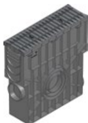
Trash box with PE mud bucket and FIBRETEC design slotted grating in the colour Black, SW 9 mm, class C 250, locked, 0,5 m
