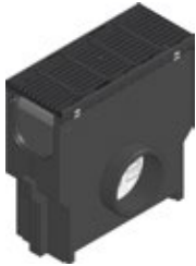
Trash box with galvanised mud bucket and longitudinal ductile iron grating SW 9 mm, KTL, class C 250, locked, 0,5 m
