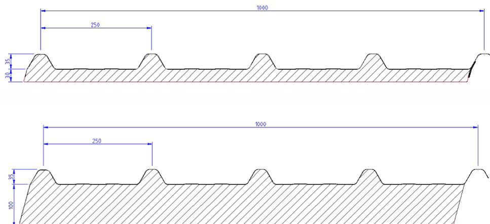
Figure 1: JI ECO PIR in thicknesses 30 mm & 100 mm
